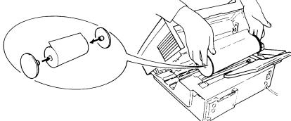
3. Pull out the leading edge about 8 ins and insert it under the green line in front of the platen roller.
